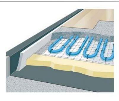
Uniformly reflects the heat from the hot water underfloor heating system back up into the room
