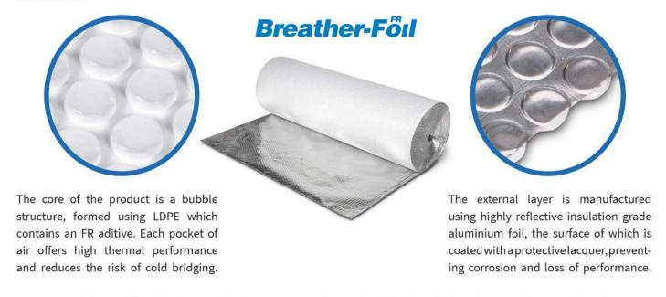
Our patented design effectivly allows timber frame constructions to breathe through the unique overlaping and venting method. Breather-Foil FR gives you a breathable and a high thermal efficent product with an over all thermal resistance value of 0.786 (m² K/W), equivalent to approximately 30mm EPS (expanded polystyrene) insulation.
